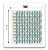
In plain weave, the warp and weft are interlaced in a basic criss-cross pattern, with the weft thread passing over the warp in an 'over and under' sequence. This results in a checkerboard style appearance which you can see if you closely examine a plain-
