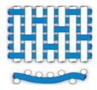
Twill is among the most widely used weaves within textile production. Easily identified by its pattern of diagonal lines, twill weave is used to create strong fabrics such as denim.
